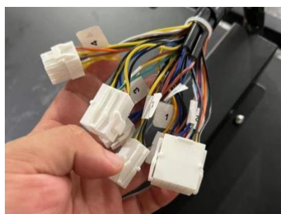
3.Just plug it in according to the numbers on the line.
