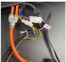
6-This flat cable (HDMI) is connected to the console's Computer at this point, Be careful not to force this connection as it could damage the output on the computer.
