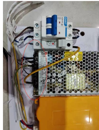
Picture 2: Power Supply Cable (Visible by opening the access door under the seat)
