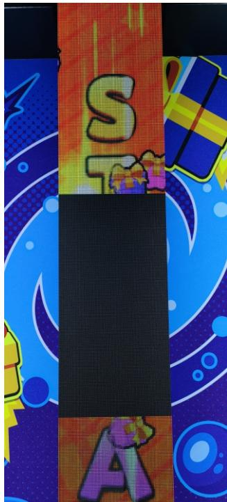
③ The voltage terminal on the dot matrix screen driver board is not connected properly or there is no 5V voltage.
